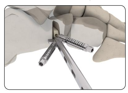
Note: A graft packing block and tamp are available to insert bone graft into the implant's graft window before insertion
